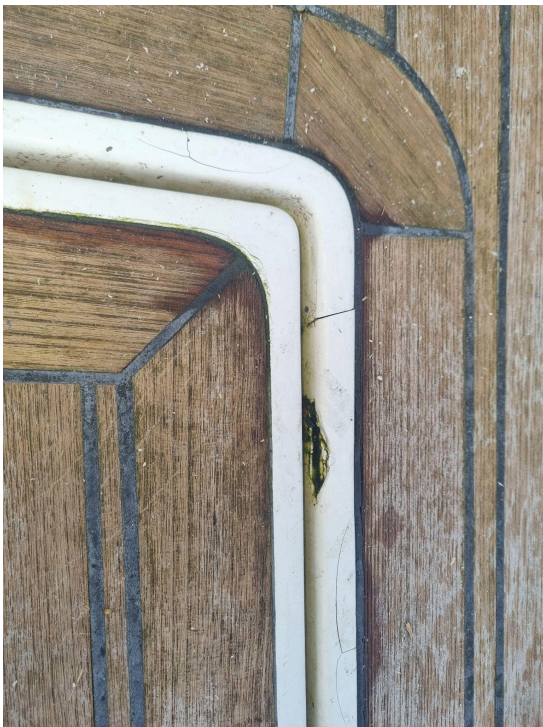
Bathing platform gelcoat damage
