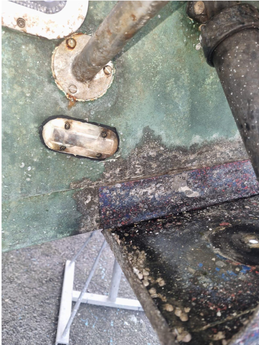
Underwater light with water in the lens
