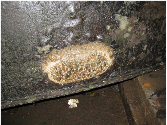
Some sample photographs showing the failure of the blacking at the waterline and the wear edge of the base plate.
