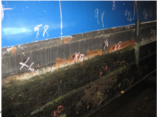
Some sample photographs showing the failure of the blacking at the waterline and the wear edge of the base plate.
